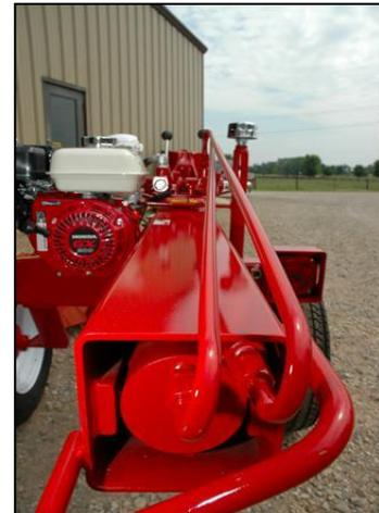
**Design:** Soft parts such as hoses, filter, and engine are well out of the way of blocks of wood being split. Seldom does wood ever get past the stop and by the time if ever it does, the wood is falling in two pieces to the ground. Moving the soft parts back also prevents damage from dropped logs when handling them.
